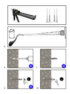
withdraw the mixer nozzle from the hole ensuring that there are no air voids as the mixer nozzle is withdrawn. Fill the perforated sleeve and withdraw the nozzle completely.
